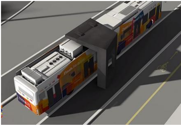
Image of Overhead Super Charger
