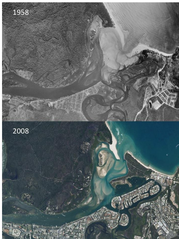
Figure 13. Aerial photographs of the Noosa River mouth, taken in 1958 and 2008 and showing the development of the Noosa Bar and Sound between the two periods. Reproduced with permission of the Department of Natural Resources and Mines.
