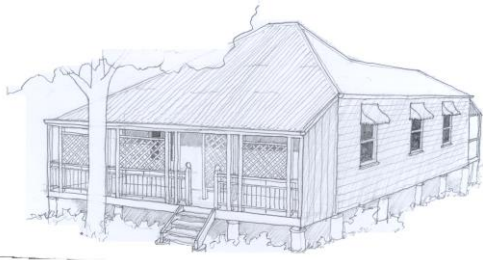
Colonial, Federation and Interwar Short-Ridge House (1870s to 1930s)
