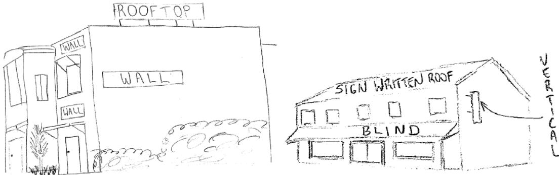
Figure 14.9 Rooftop, Wall, Sign Written Roof, Blind and Vertical Signs
