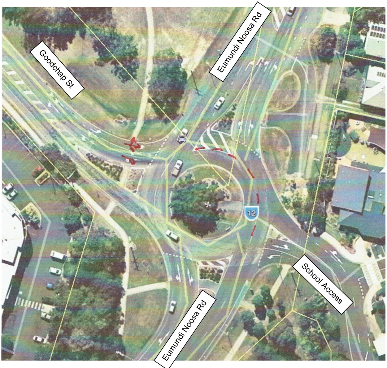
Figure 30: Recommended alteration to the Goodchap Street / Eumundi Noosa Road intersection
