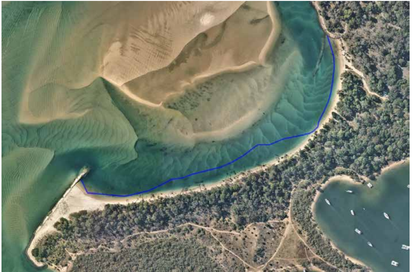
Figure 2: Current day (June 2019) aerial image with the June 2013 shoreline position shown in blue, showing the progressive erosion over this six year period. Image: Nearmap (2019).
