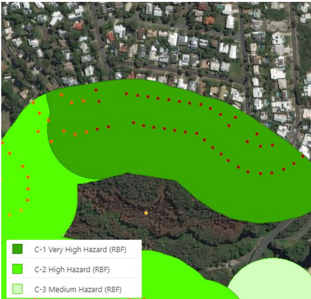
Map 4. An example of Bushfire Interface Zone mapping. The green areas are the 100m Bushfire Interface Zone in relation to vegetation and buildings (shown as dots). (Source: Qld Gov.)
