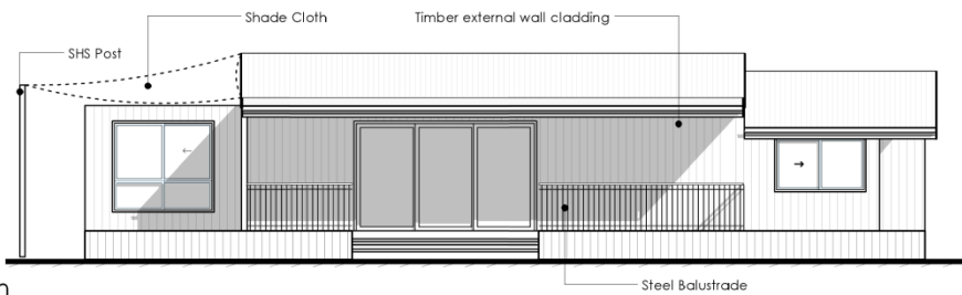
Elevation North West Elevation 1 : 100
