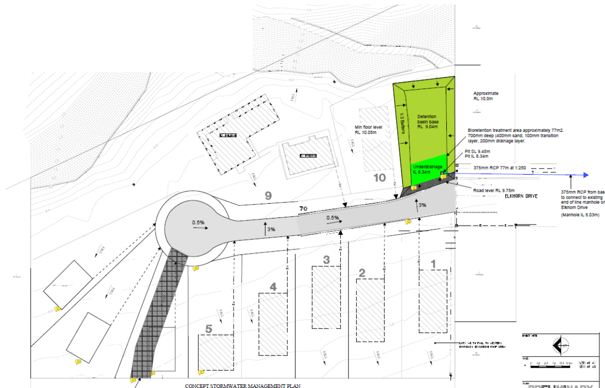
Figure 3 – indicative location of stormwater solution
