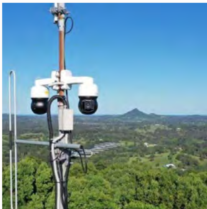
Ultra high-definition cameras being used to detect fires early, verify their location and provide real time intelligence
